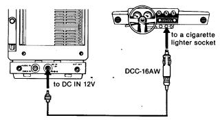
• The DCC-16AW is designed for use with a 12V negative ground system.
